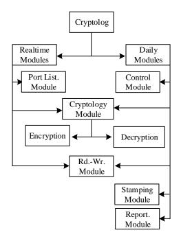
Figure 1. Overall structure of the proposed system
